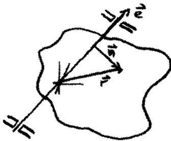
$\vec{v} = v \cdot (\vec{e} \times \frac{\vec{r}_\perp}{r_\perp}) = \frac{v}{r_\perp} (\vec{e} \times \vec{r}_\perp)$
