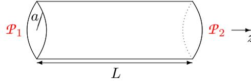
**Figure V.3** – Setup of the Hagen–Poiseuille flow.
