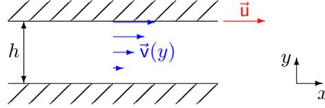
**Figure V.1** – Setup of the plane Couette flow.
